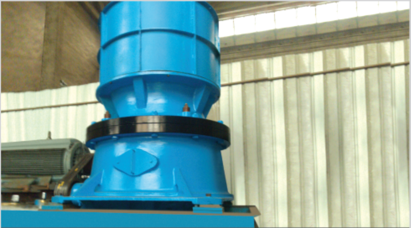
Cone Crusher | For Crushing Moderately Hard to Hardest Rock
